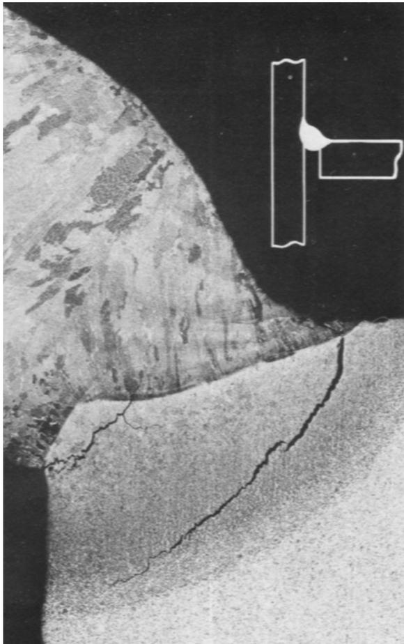
**Hydrogen induced cracking is influenced by factors such as high hardness in heat affected zone (HAZ), high residual stresses, and rapid cooling which does not allow hydrogen to diffuse out**
