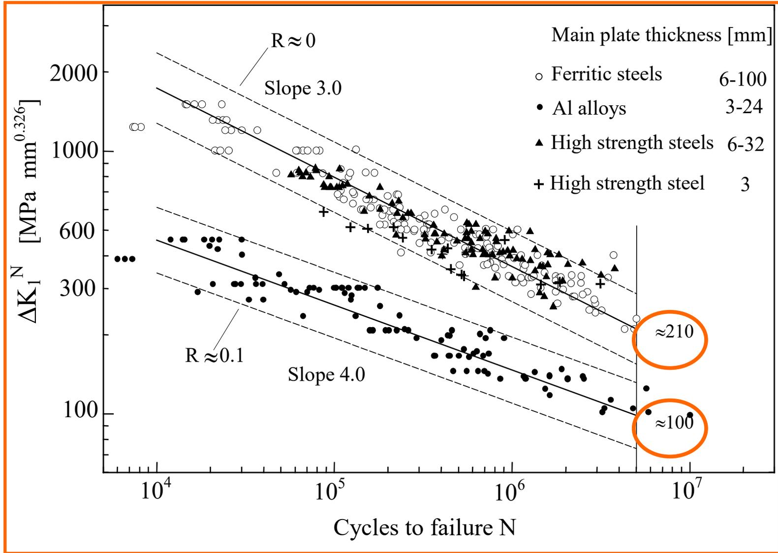
Fatigue strength of steel and aluminum fillet welded joints in terms of the Mode I NSIF (Lazzarin and Tovo 1998, Lazzarin and Livieri 2001). Scatter bands defined by mean values of  $\pm 2$  standard deviations.
