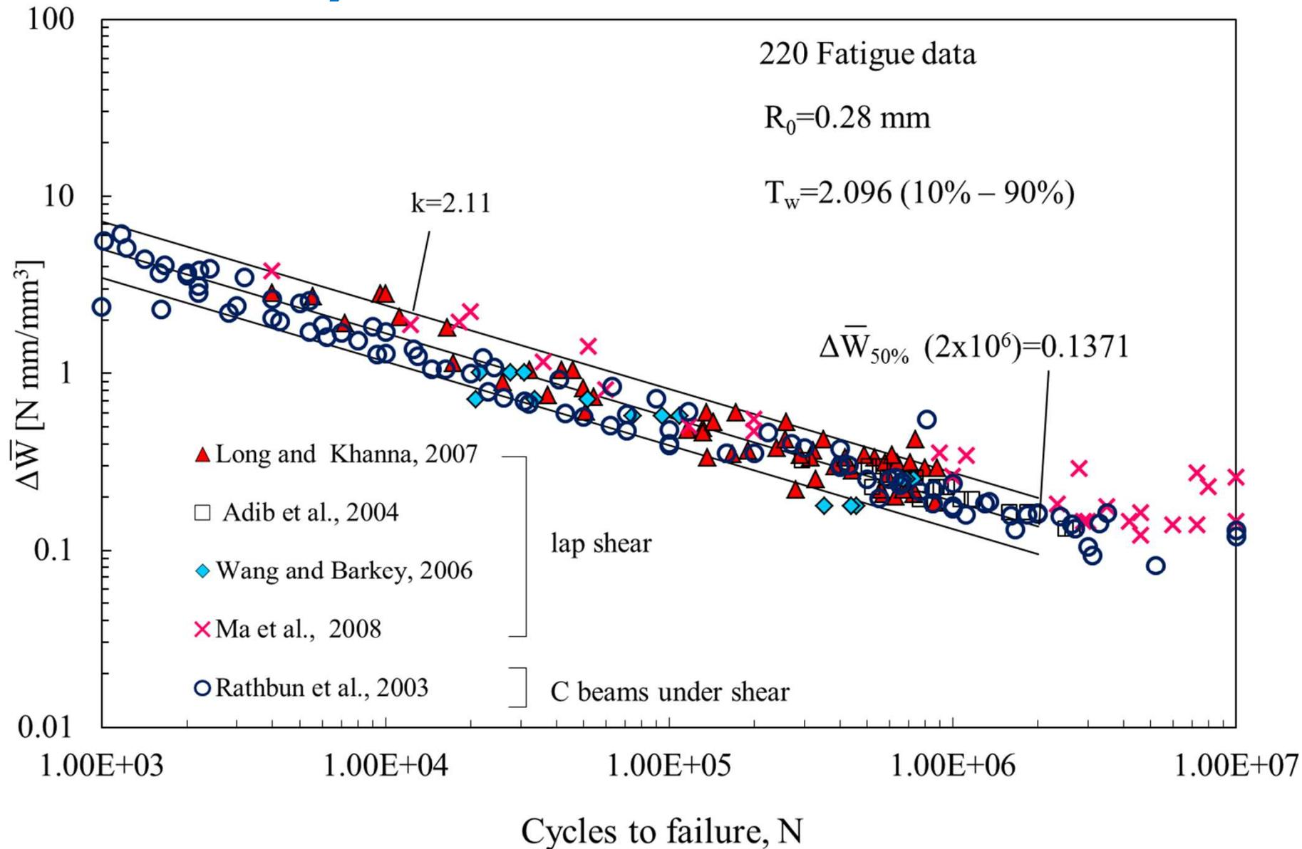
Synthesis of data from spot-welded joints under tension and shear loading. The thickness  $t$  ranges from 0.65 to 1.75 mm. SED values have been determined by means of three-dimensional models. The control radius of the toroidal volume is equal to 0.28 mm
