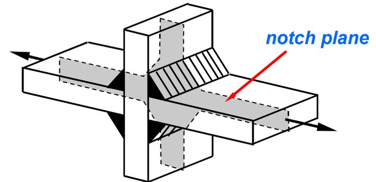
“Real” geometry at the weld toe
