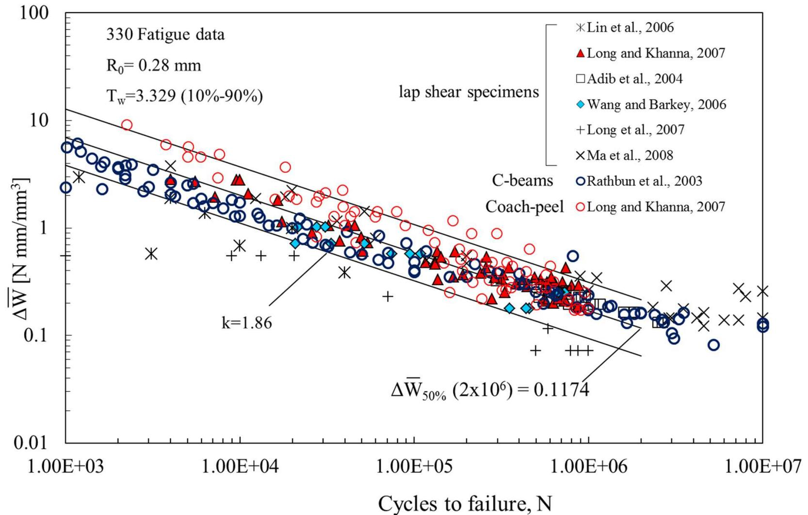
Synthesis of data from lap shear specimens, C-shaped specimens and coach-peel tension specimens (330 data,  $TW=3.32$ )
