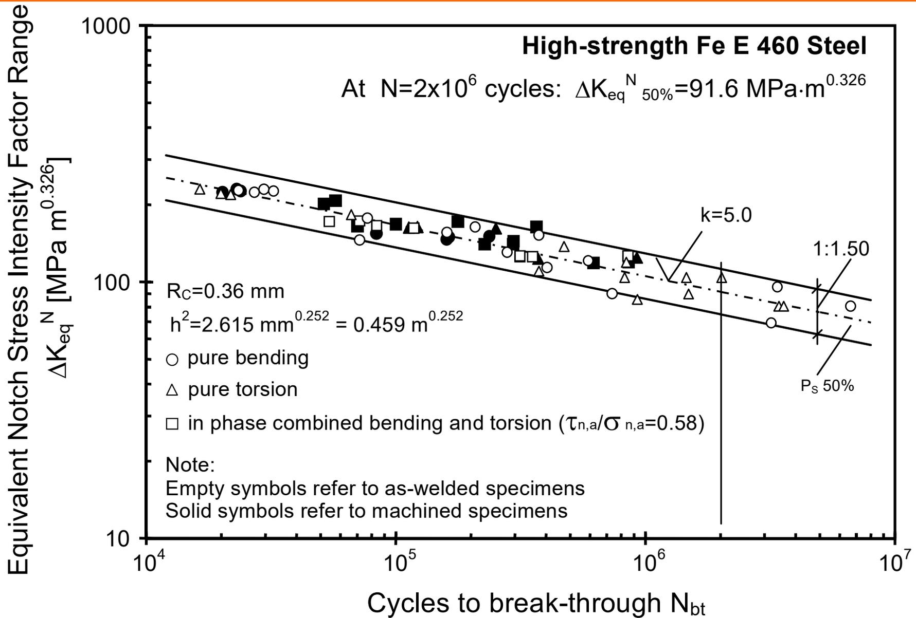
Figure 40: Fatigue test results related to as-welded and machined specimens [33-35].
