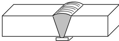
Butt weld made from one side on a backing bar
