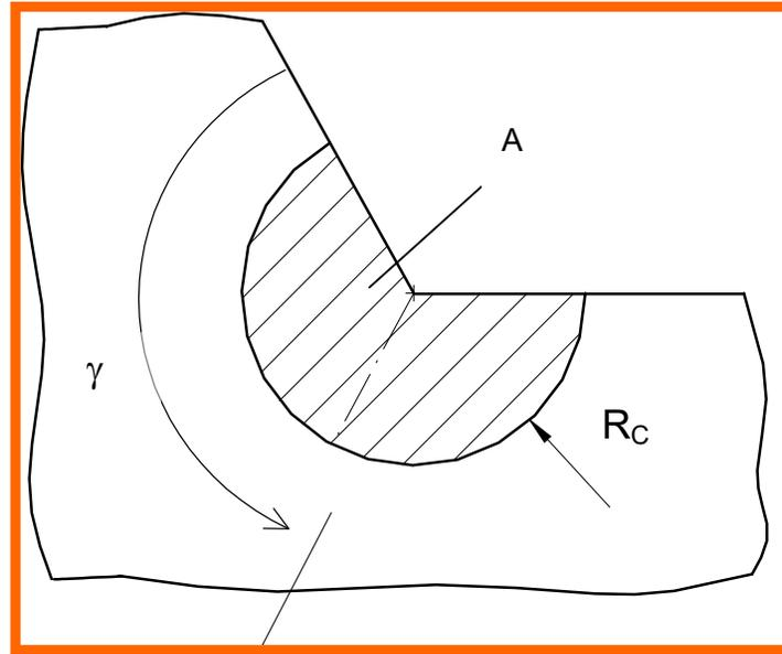
**The critical value of the radius  $R_C$  mainly depends on the material. The more brittle is the material, the smaller  $R_C$  is**
