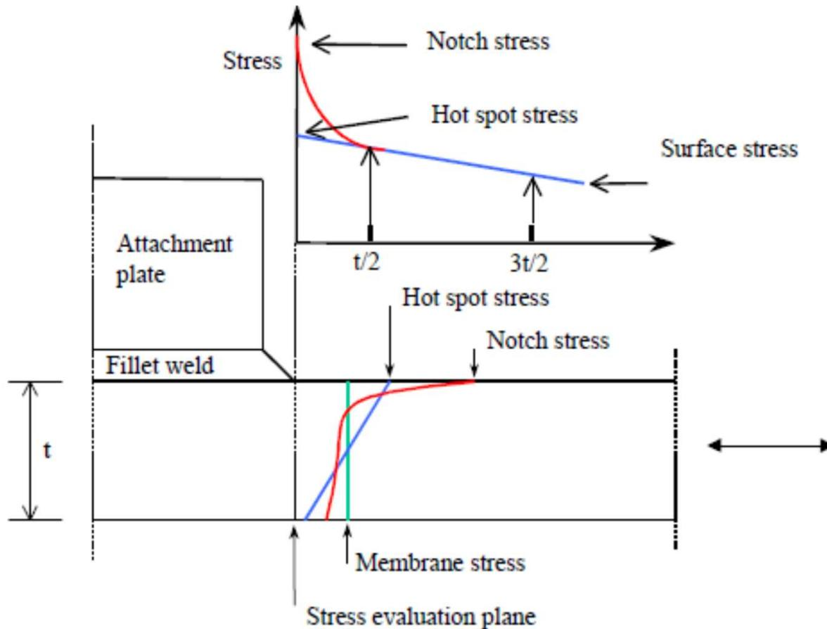
The hot spot stress is a linear extrapolation at distances  $0.5t$  and  $1.5t$  from the weld toe.
