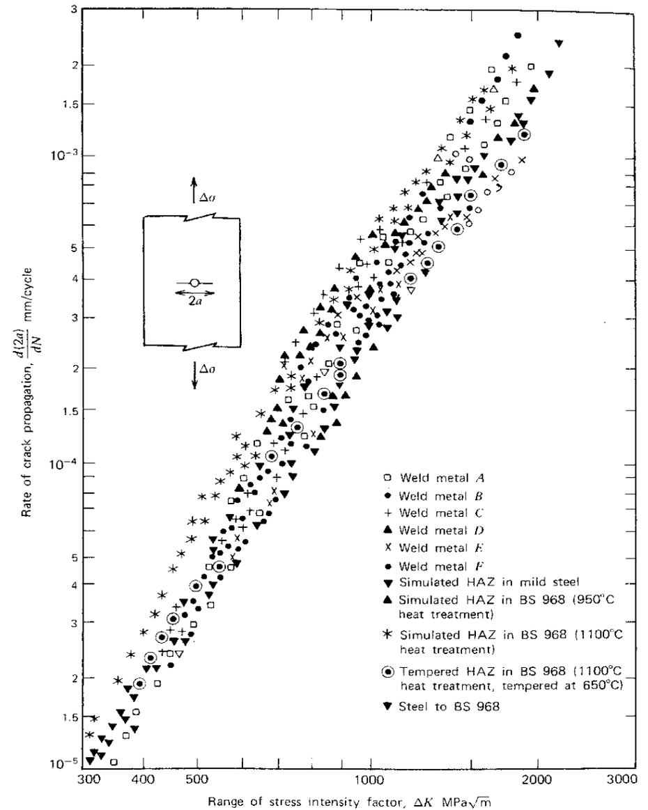
Crack growth speed is almost independent of steel strength therefore the fatigue strength of welded joints is the same for low and high strength steels, in contrast to machined components
