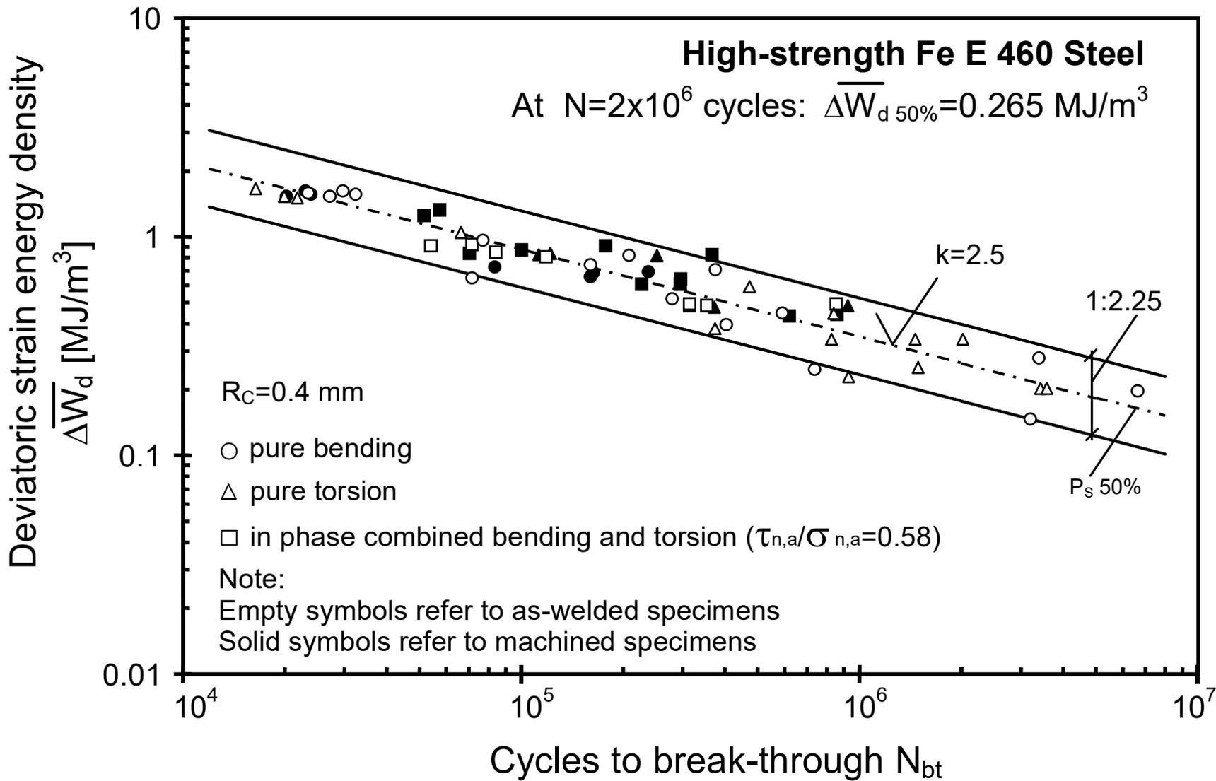
Fatigue test results related to as-welded and machined specimens in terms of the mean value of the strain energy density range. Nominal load ratio  $R = -1$
