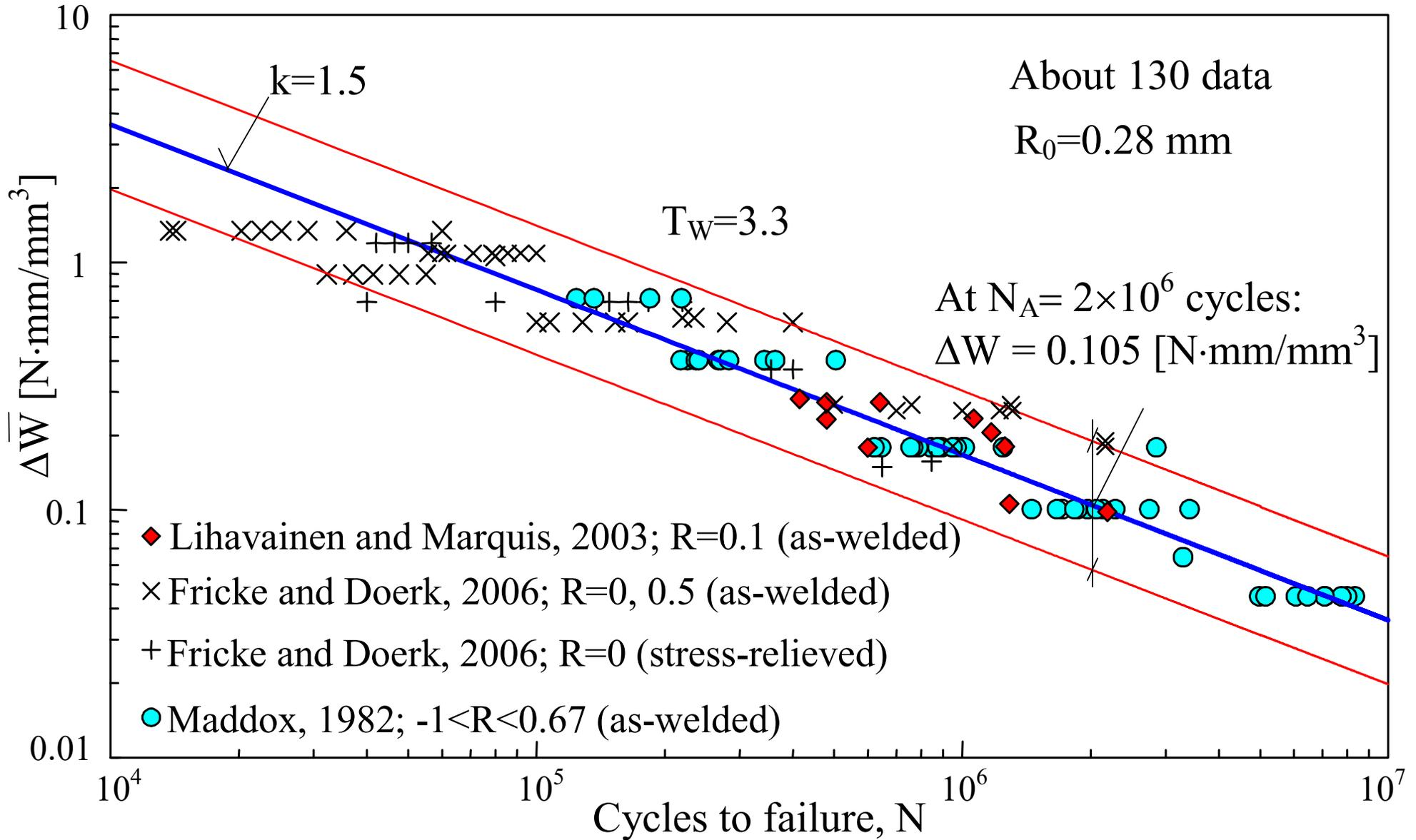
**Fatigue strength of the welded joints made of structural steel in terms of local strain energy density; comparison with the scatter band previously proposed**
