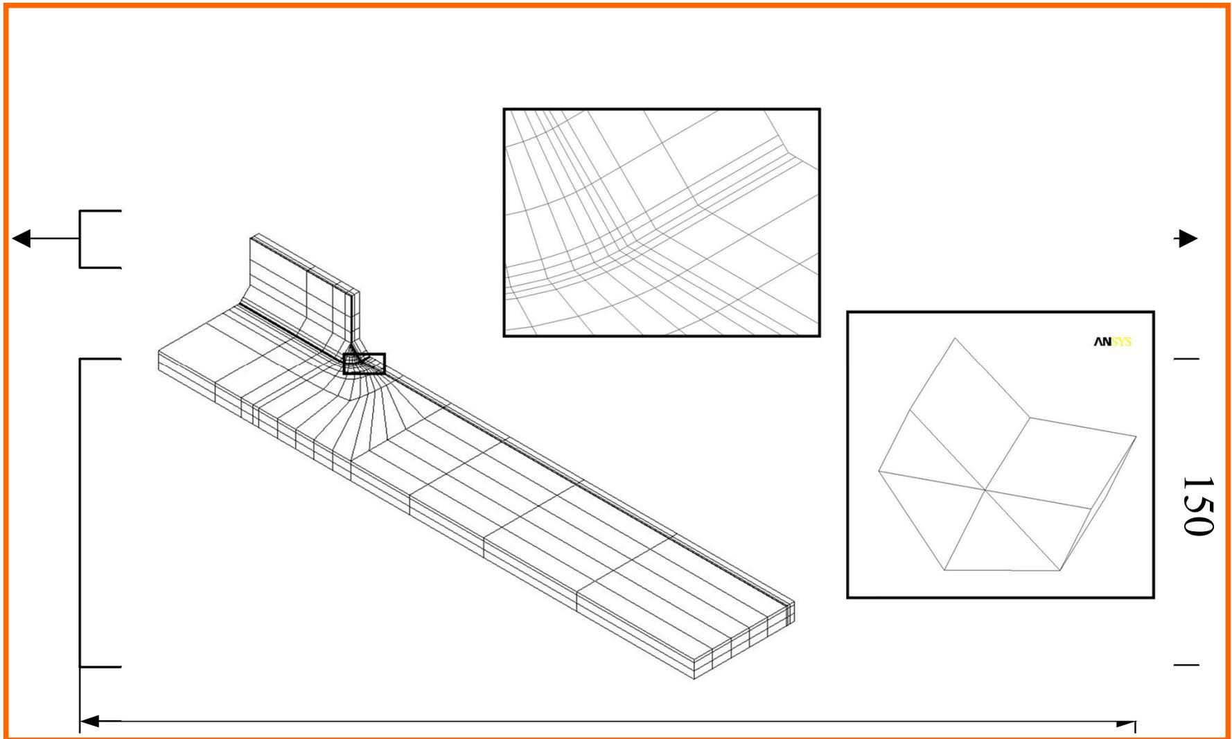
**Geometry of the welded joints with a longitudinal stiffener tested by Maddox**
