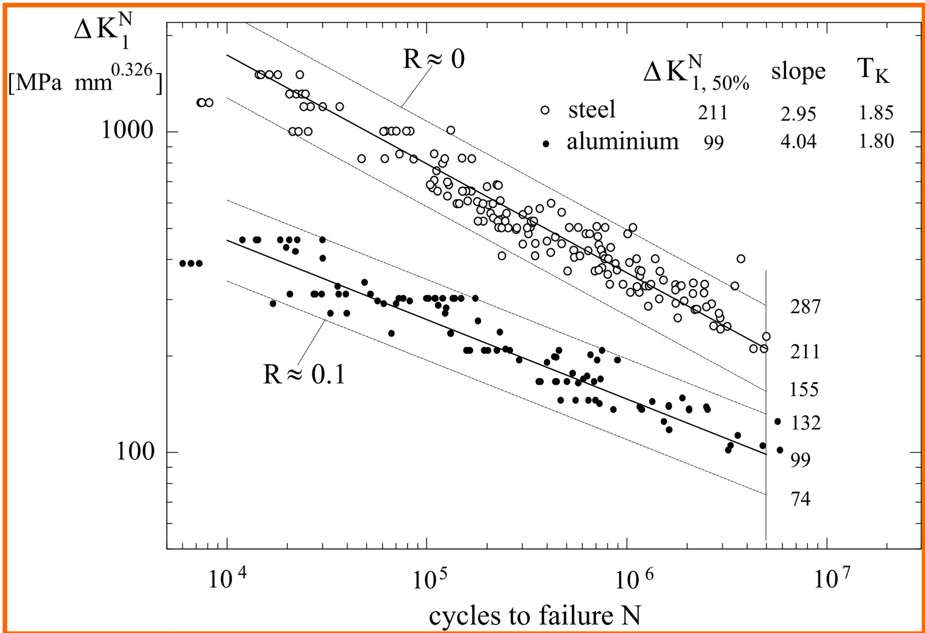
Fatigue strength of aluminium and steel welded joints as a function of Mode I Notch Stress Intensity Factor. Scatter band related to mean values plus/minus 2 standard deviations
