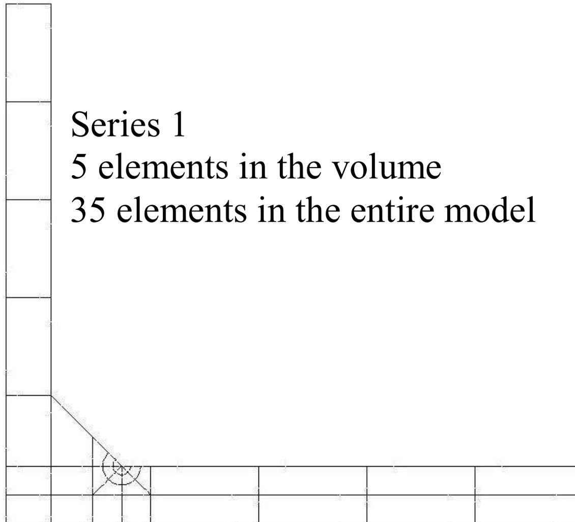
The SED can be accurately evaluated by using coarse meshes.
