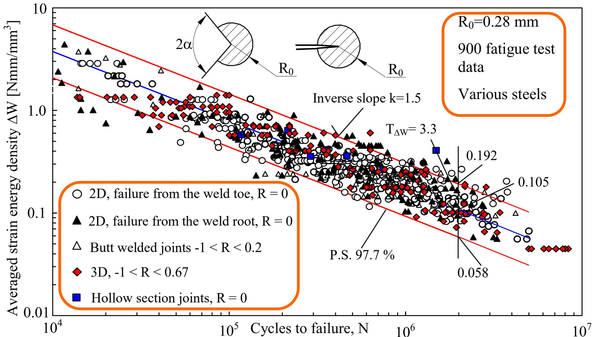
Fatigue strength of welded joints as a function of the averaged local strain energy density;  $R$  is the nominal load ratio (Berto and Lazzarin 2014)
