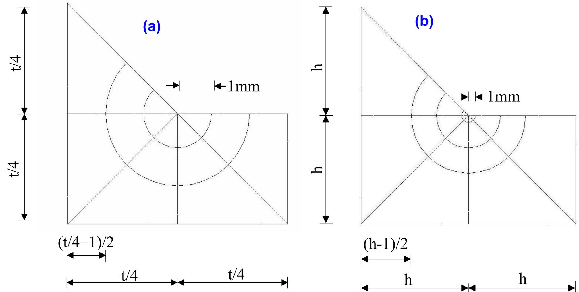
Modulus used for the geometries with  $h > t/2$  (a); modulus used when  $h < t/2$  (b)
