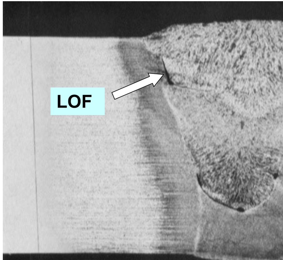
**Lack of fusion is caused by e.g. too low current or incorrect torch angle.**
