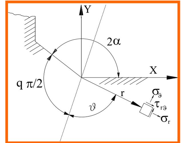
Coordinate system and geometrical parameters for the analyses of the welded joints
