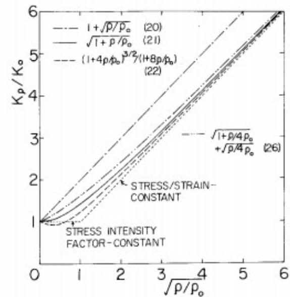
Figure 4. Effect of notch-tip radius on critical stress intensity.
