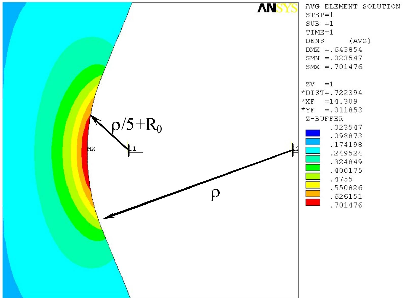
The SED contour lines are parallel to the volume perimeter
