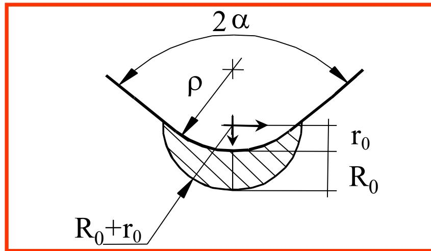
The criterion based on the local energy and valid for brittle or quasi-brittle material considers that the strain energy averaged over a control volume is critical for notched components
