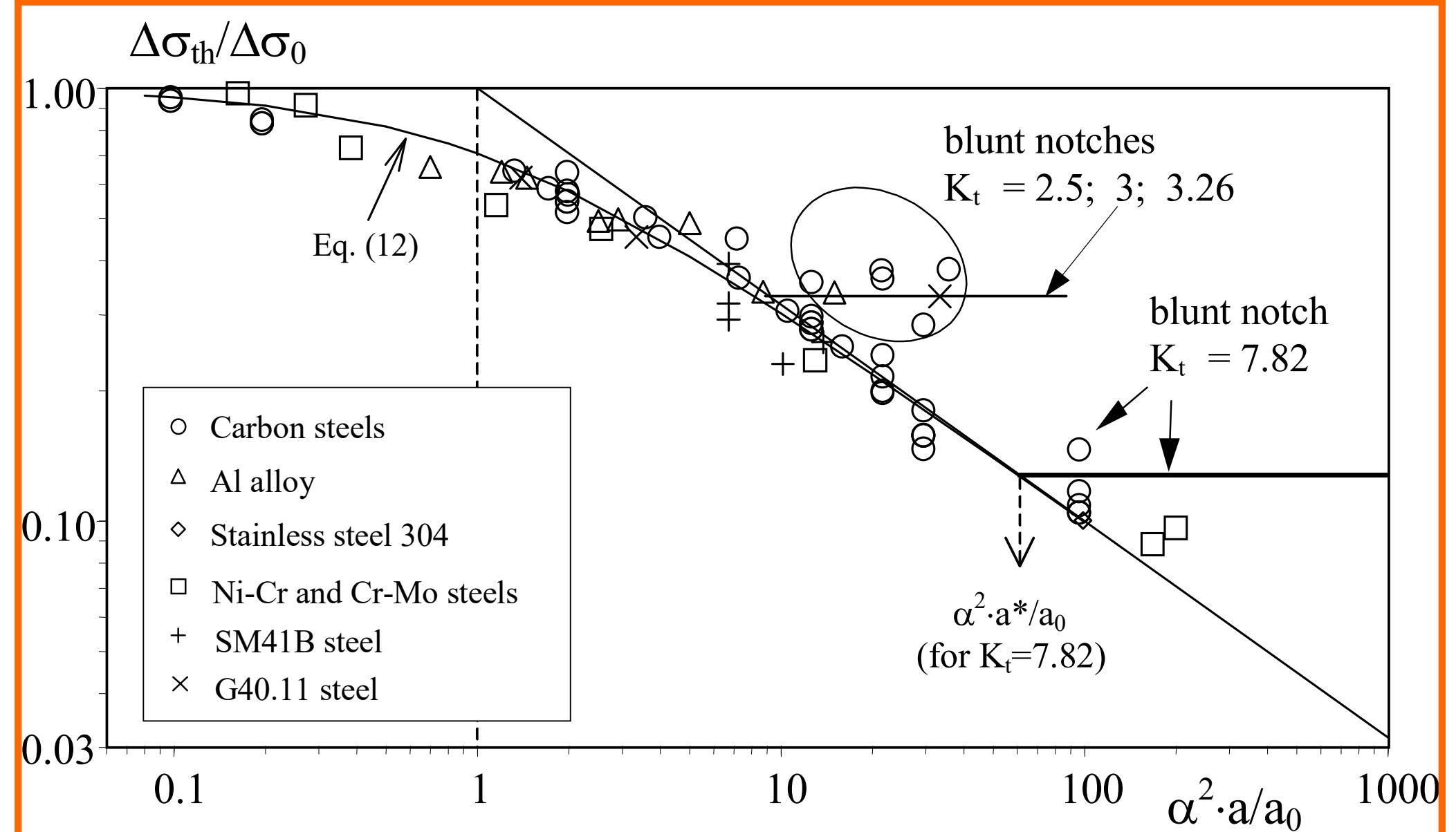
**Fatigue strength of specimens containing defects and notches**
