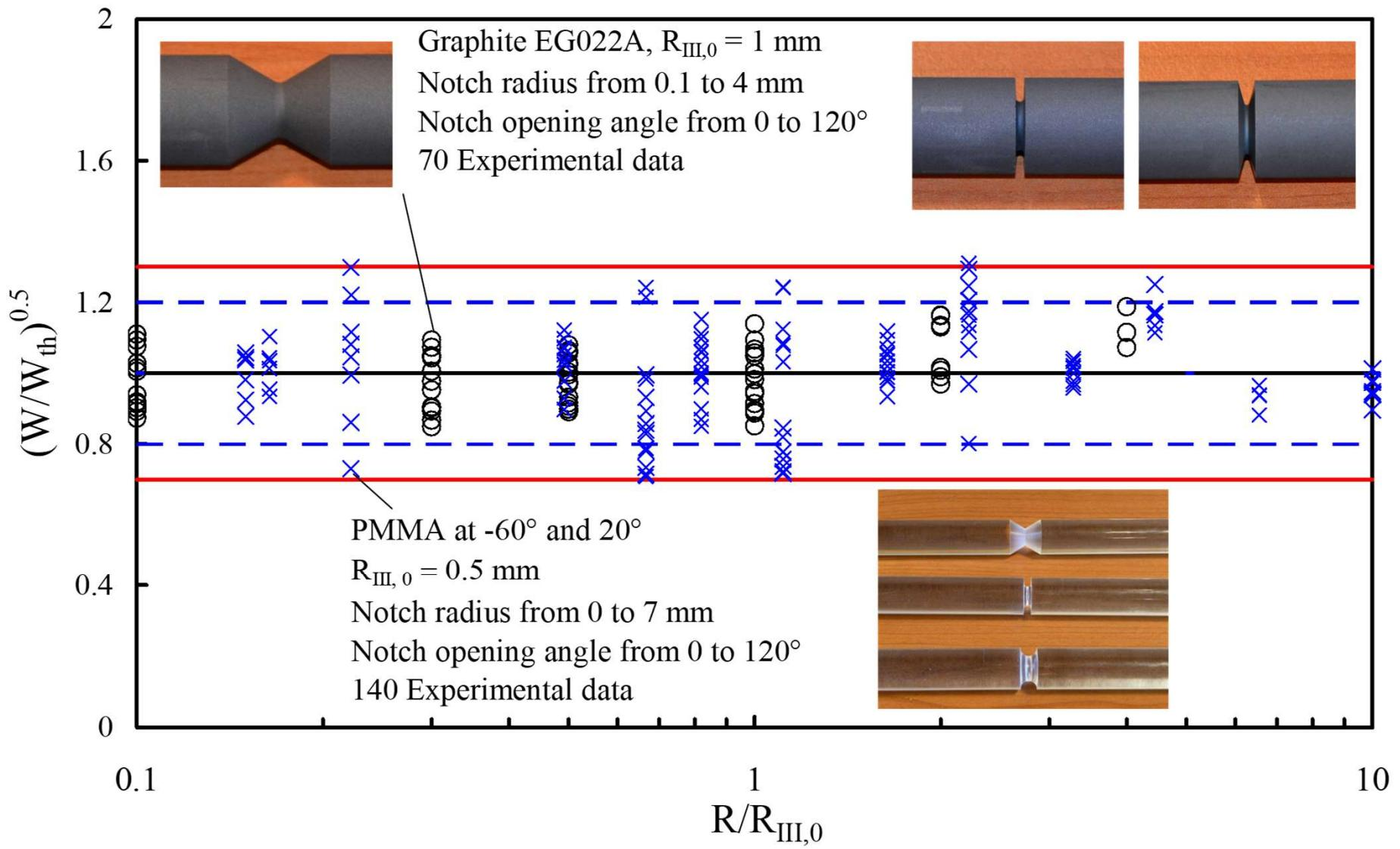
Synthesis of 210 new data from notched specimens under torsion
