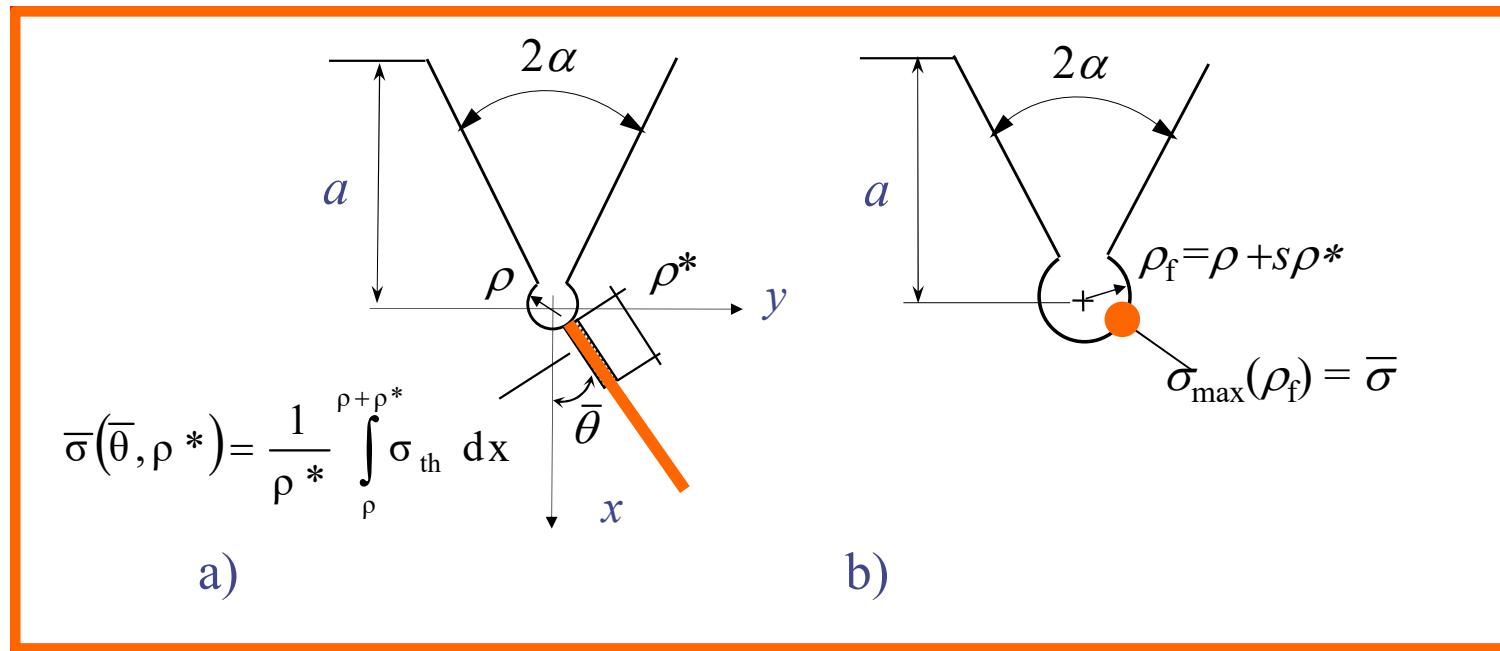
**Method 2:** Neuber's approach, by using the analytical frame for notches with "end holes at the tip" and evaluation of the fictitious notch radius (normal stress only)
