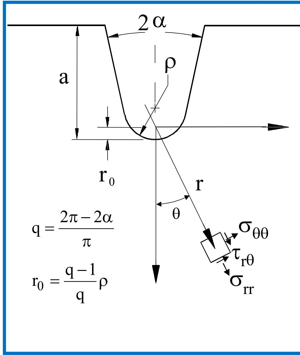
**Coordinate system and symbols used for the stress field components.**
