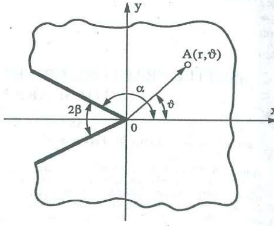
Fig. 1. Notch geometry in polar coordinate system.
