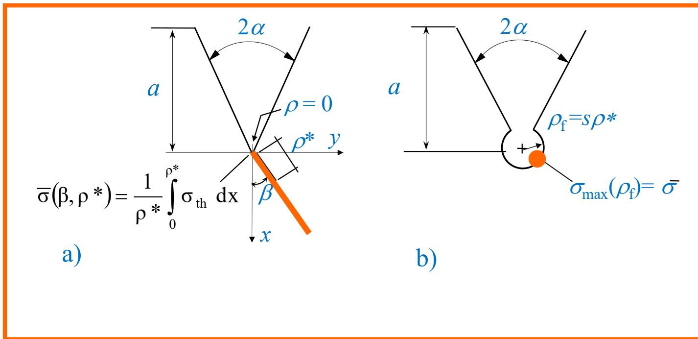
**Method 1:** direct comparison between the mean stress obtained by a sharp V-notch along the direction of provisional crack propagation (Sih, Erdogan-Sih) and the maximum stress along the edge of the notch with radius  $r_f$  (normal stress, von Mises, Beltrami, plane stress e plane strain)
