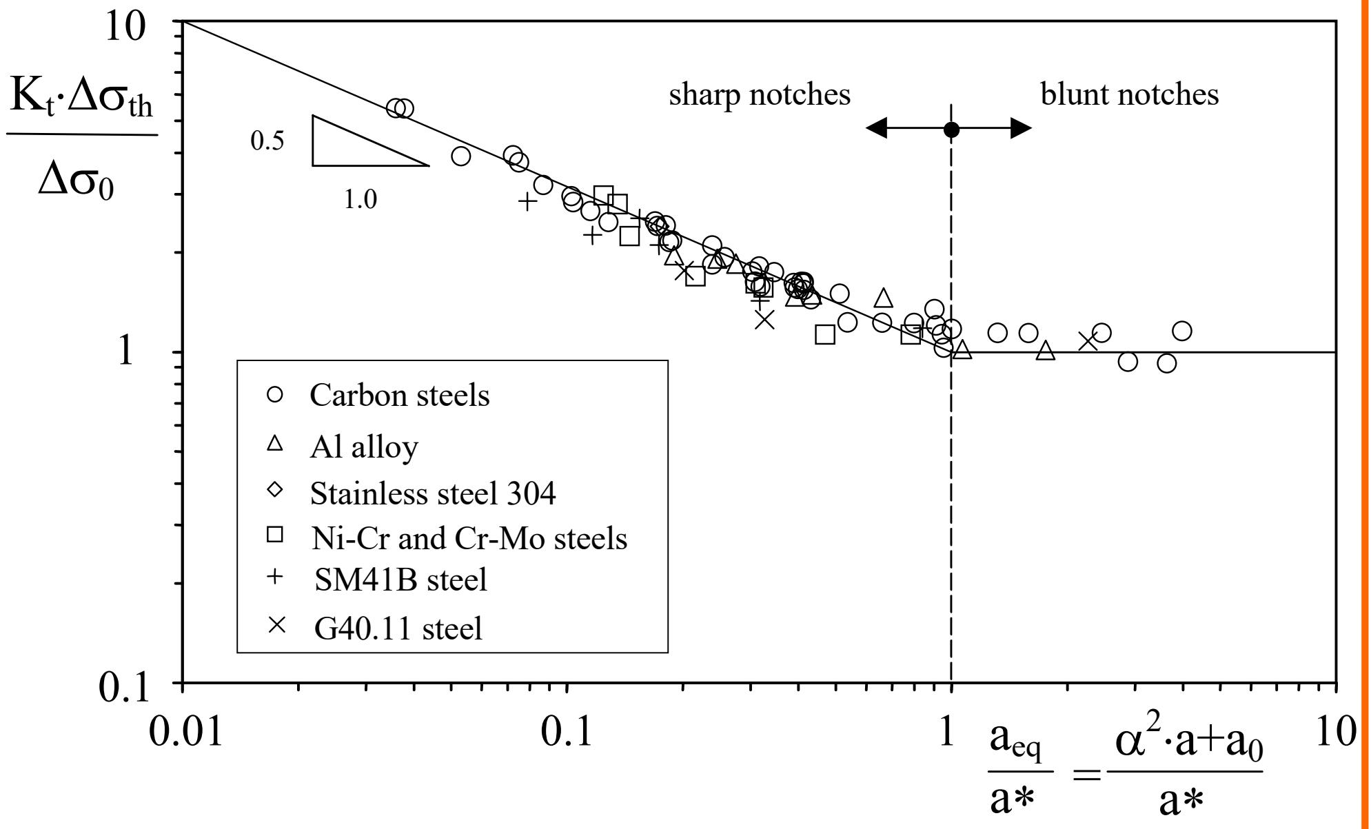
**Transition between the fatigue behaviour of sharp and blunt notches versus the equivalent notch size normalised with respect to  $a^*$ .**
