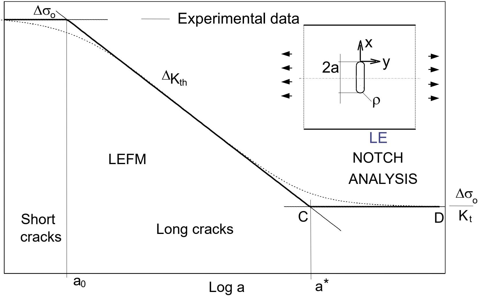
**Fatigue behavior of a material weakened by notches or cracks**
